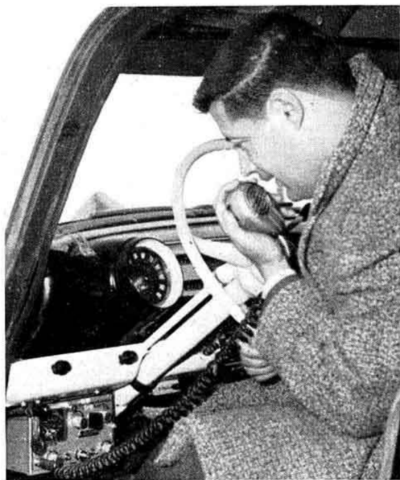
VE2ACT/M operates on 28-256 Mc/s phone, usually between 1800 and 1900 G.M.T. daily. The transmitter, a crystal controlled Babcock, runs 18 to 20 watts input. The aerial wire runs under the car to a whip at the rear. More than 70 countries have been worked. The regularity of operation of VE2ACT should be useful to I.G.Y. observers in connection with the H.F. Project.
