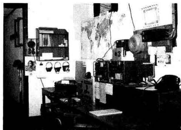
This is the operating position at VS1HU, station of the Kranji Amateur Radio Club, Singapore. Equipment visible includes a TCS transmitter-receiver for 7 Mc/s and a CR100 receiver with "S" meter standing on top. The main transmitter, running 100 watts to an 813, is situated out of the picture to the left. The aerials are a 300 ft. long wire and a 7 Mc/s dipole. The Kranji Club was founded by Mike Matthews (G3JFF).
